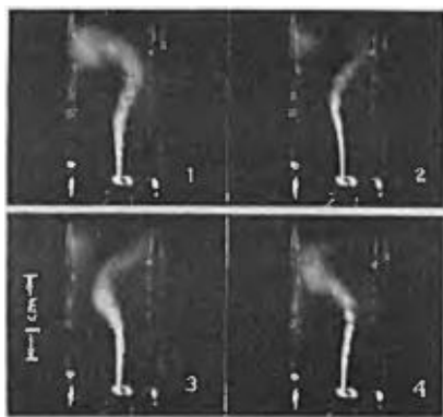
FIG. 6. Snapshots of jet in sound field. Four frames \frac{1}{4} cycle apart in time. Blowing pressure 1.0 in., initial jet velocity 1920 cm sec -1 . Acoustic peak particle velocity 38 cm/sec.
